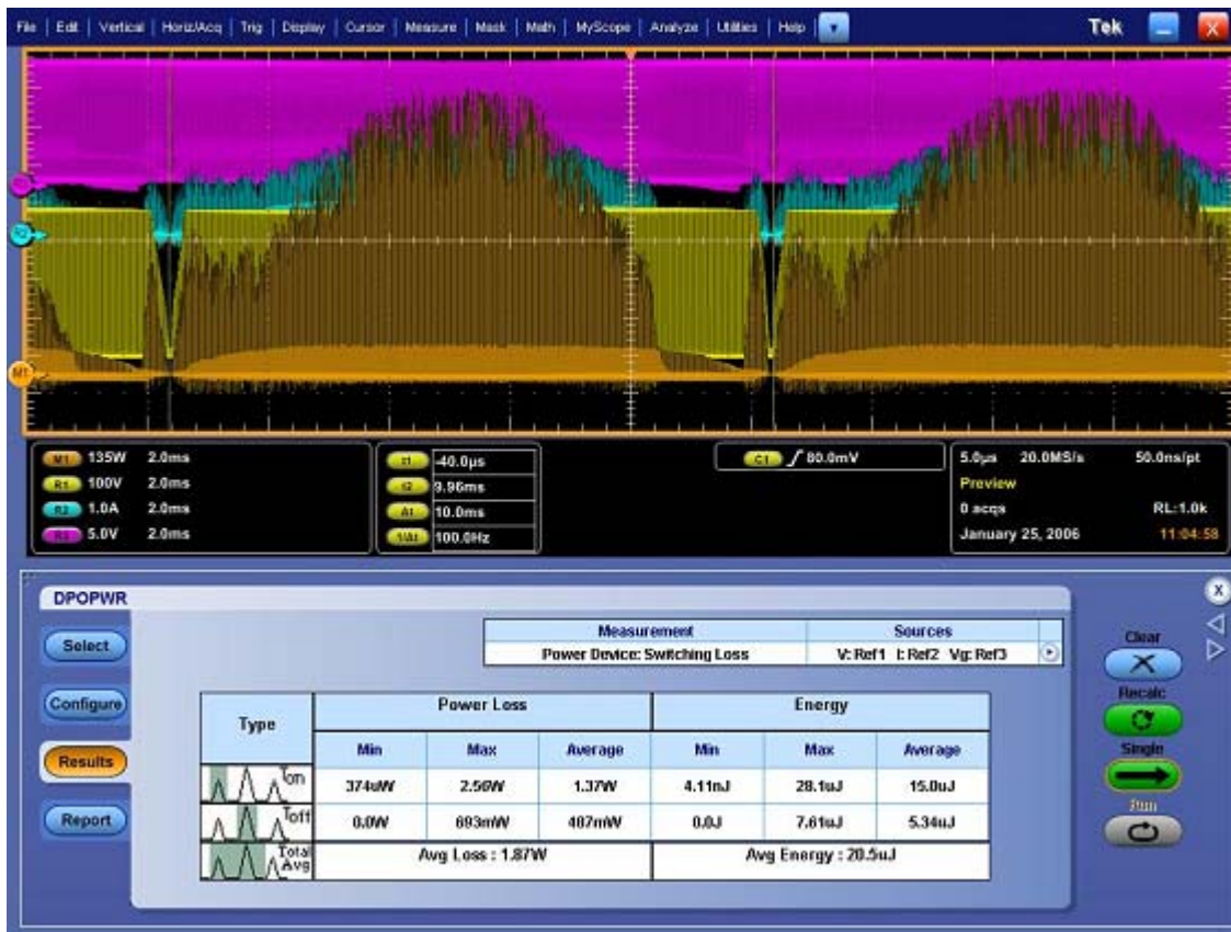
Figure 21: Switching Loss results
