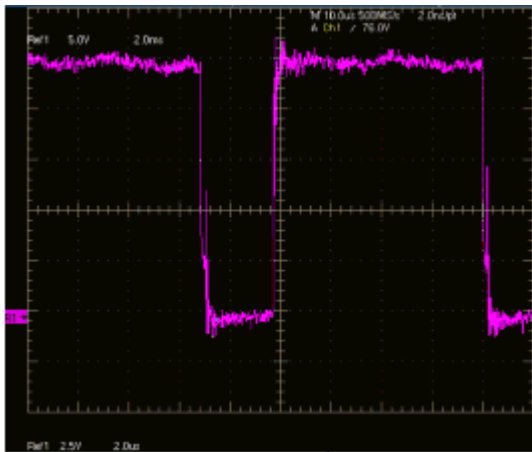
Figure 24: Gate signal without a glitch
